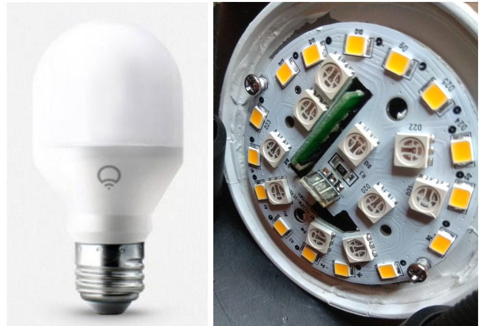
Left: LIFX Smart Bulb. Right: Tuya smart bulb with cover removed.
