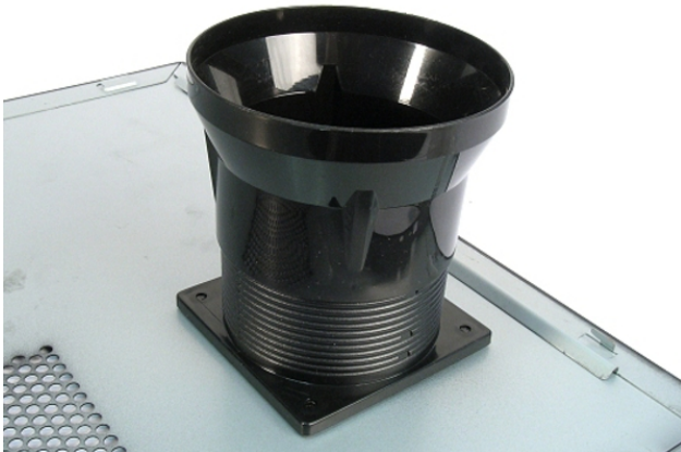
a typical CPU duct shown mounted to the side panel of a case
